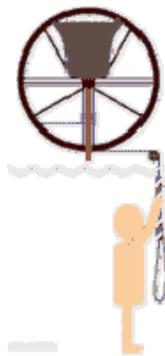
In a change ringing room, the ringers stand in a circle, one behind each bell rope. Students can see in this [one bell animation](#) how a bell is rung 'full circle' by pulling on, and then releasing, the bell rope.
